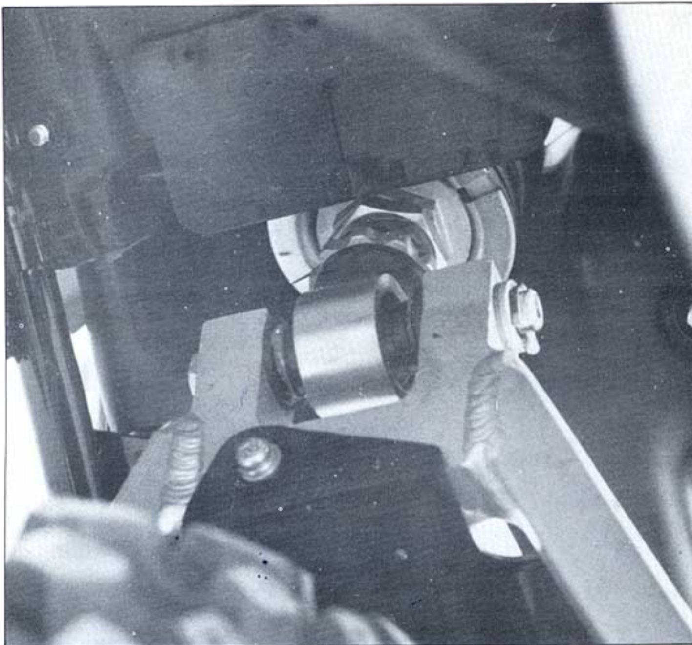
Changing the mono's damping characteristics is as easy as turning a knob.
