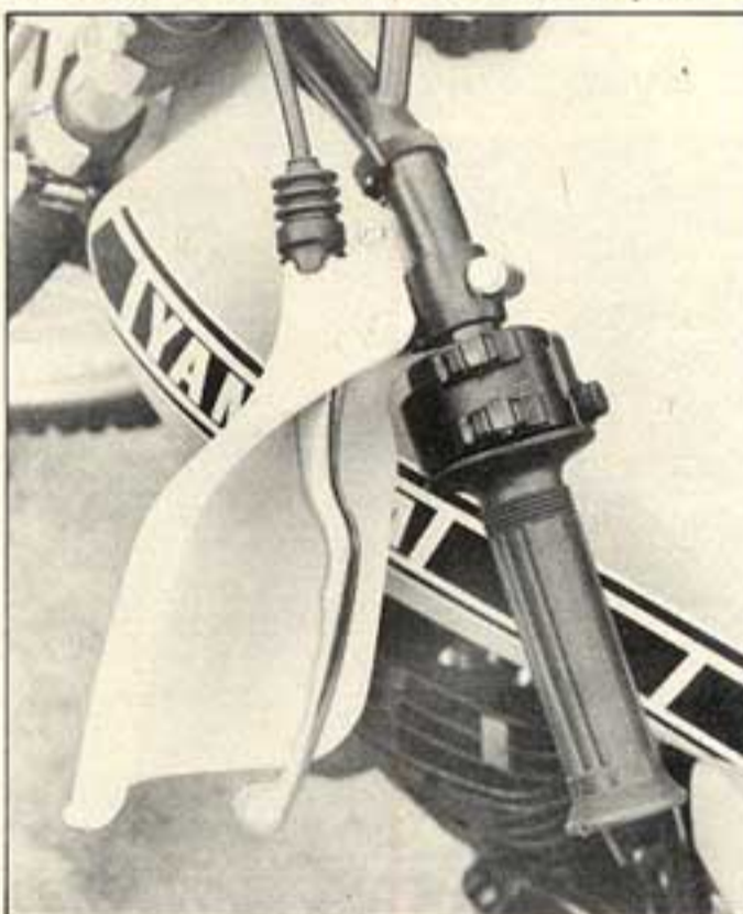
Handlebar brush guards are useful in tight situations, and easily removable for anything else.
